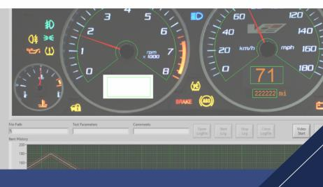
The ICE system uses a video camera to monitor the different indicators and displays on an instrument cluster (or any other device).
